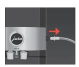
If insufficient foam is produced when the milk is frothed or milk sprays out of the dual spout, the spout may be dirty. If this happens, dismantle and rinse the dual spout.
